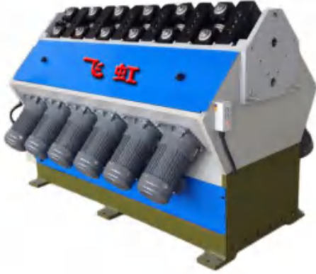
Popular reducing machine in the market Center distance: 105mm 市场通用型缩管机 中心距: 105mm
